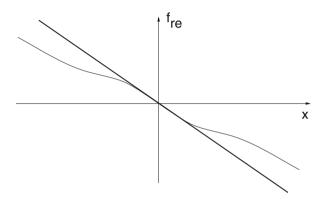
Fig. 10.7 Linearized restoring force
