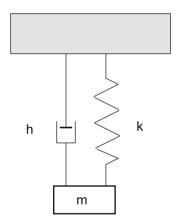
**Fig. 10.13** A spring and mass with friction. Before gravity is applied, y = 0 is the equilibrium.  $f_{\text{re}}(y) = -ky \ f_{\text{fr}}(v) = -hv$ . See Problem 10.20
